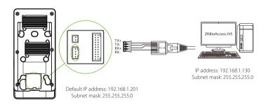
Click [COMM.] > [Ethernet] > [IP Address], input the IP address and click [OK].
